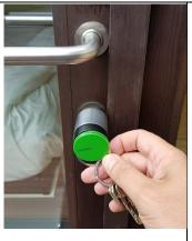
To open the door hold the tag to the reader for a few seconds untill it beeps, then turn the knob to unlock
